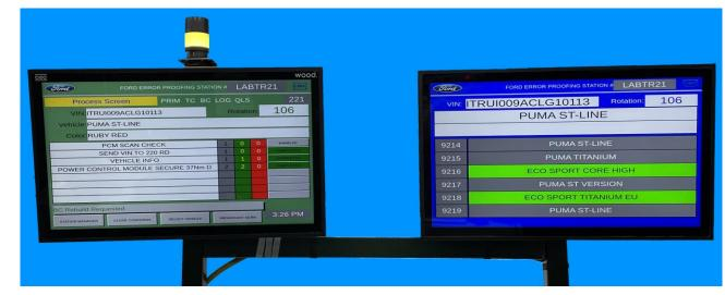
Tracking Controller with Live line view showing line status, vehicles on the line, AIS Stations statuses, live view of AIS screens
